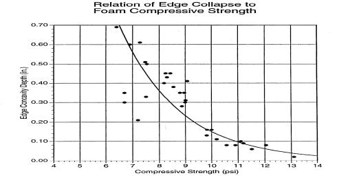
Figure 7 Edge Collapse Relative to Foam Compressive Strength at the Edge
