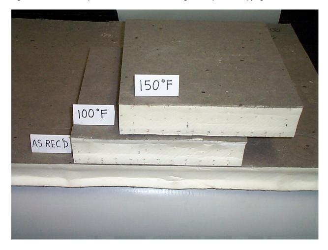
Figure 8 Effect of Temperature on Boards with Edge Collapse or Cuppage
